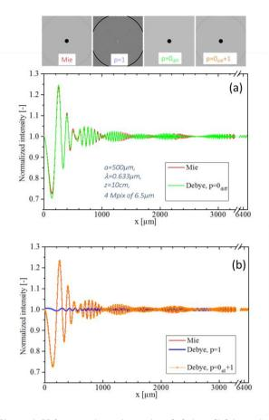
**Figure 2** Holograms (gray images) and their radial intensity profiles when all scattering processes are taken into account (Mie), only pure diffraction ( $p=0_{diff}$ ), only single refraction (p=1), single refraction and reflections ( $p=0_{all}+1$ ). Water droplet in air ( $k_{aa} = 4963$ ).
