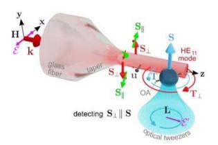
**Figure 1** Schematic of the experiment for a demonstration of the transverse spin of light. An anisotropic particle is trapped using an optical tweezers and placed in the evanescent field of an optical nanofibre. An optical torque  $\mathbf{T}_{\perp}$  is produced via the transverse spin of light  $\mathbf{S}_{\perp}$  and this contributes to the total torque  $\mathbf{T}$  on the particle [9].
